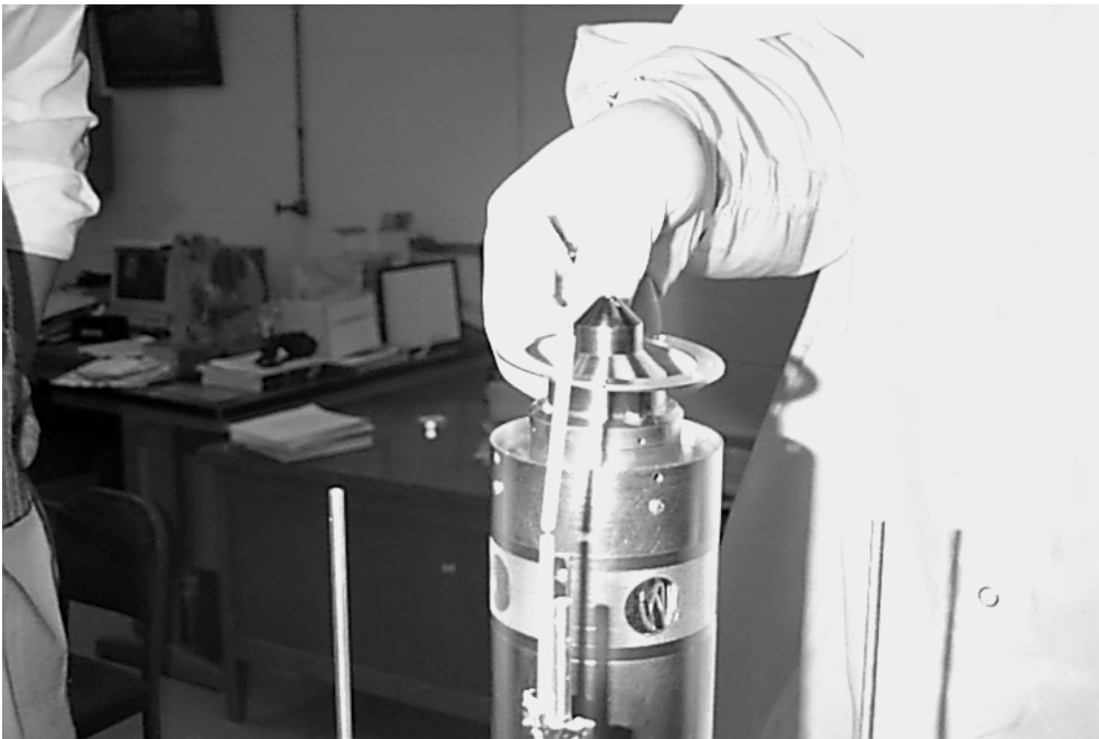
17. Remove the 4 pan head screws on the upper part of the inner cylinder.
