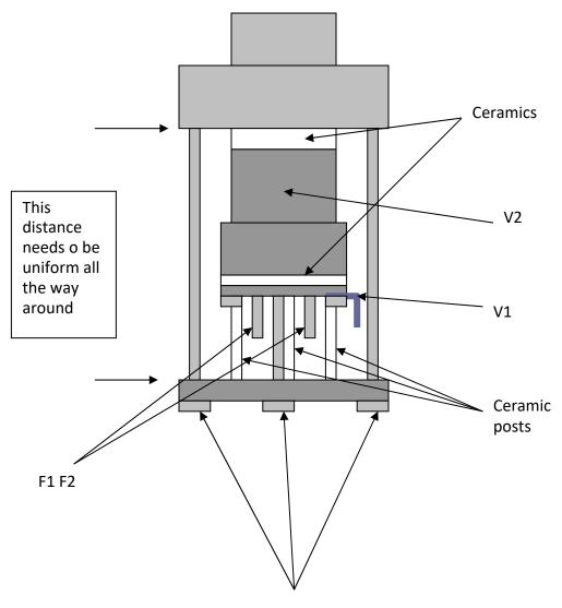
These screws hold the gun assembly together. It is stacked on the ceramics. Tighten it up, but not too much. All 3 screws should have the same distance with-in .001".
