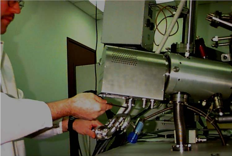
2. Disconnect the differential pumping line. Protect the knife-edge with aluminum foil.
