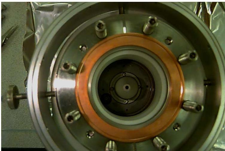
13. Remove the 4 screws, which hold the intermediate electrode to the base of the source and lift out the intermediate electrode.
