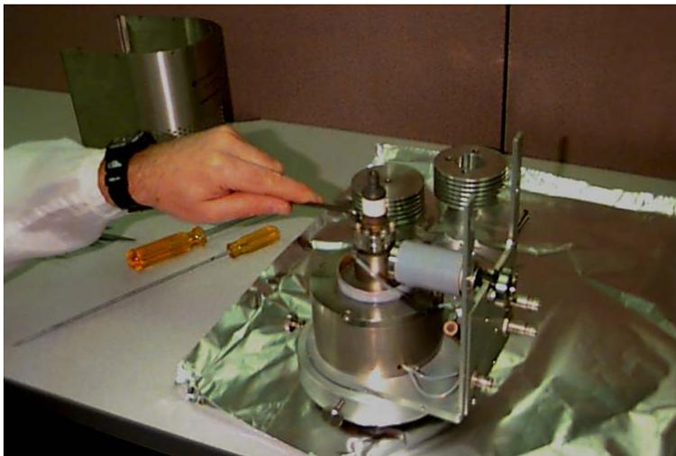
9. Remove the cathode ceramic by lifting it straight up. Tip: make a lip on the edge of the aluminum foil to capture the red sapphire beams which will fall out when the cathode ceramic is removed. These sapphire beads insulate the cathode from the intermeditate electrode. (You can clean the nickel off of these beads with a small amount of diluted nitric acid and re-use them if you have access to a chemistry lab).
