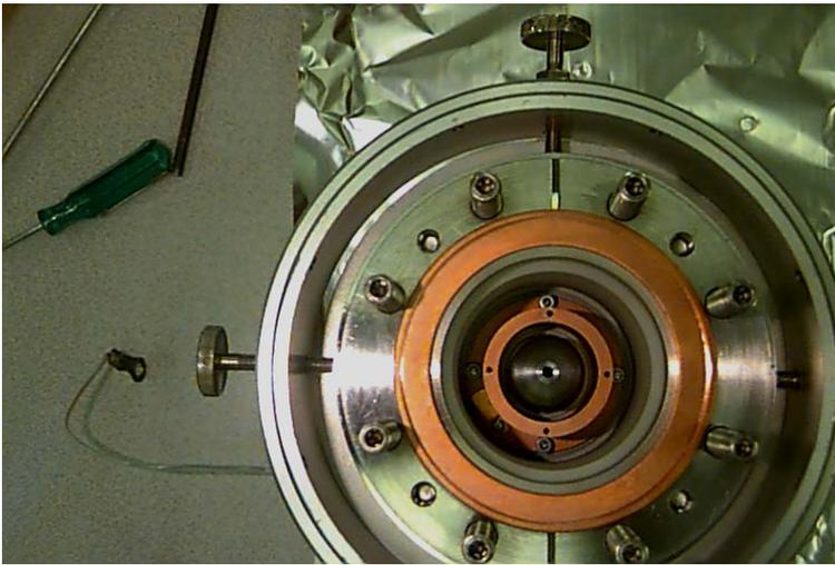
11. Remove the 4 screws (also the washers and ceramics) that hold the anode support to the base of the source. Use a needle nosed pliers to lift the screws and washers out.
