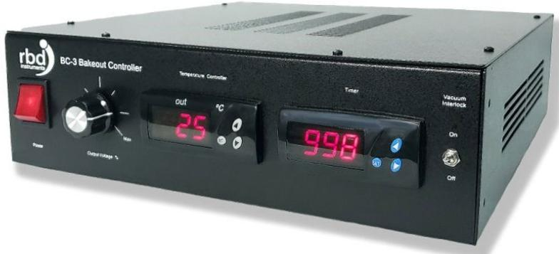
1. Place the BC-3 controller where you will be using it. 19" rack adaptor brackets and hardware are included if mounting into a standard electronics rack.
