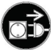
This symbol indicates that the equipment must be unplugged from its power source before any service or maintenance is performed on the equipment.
