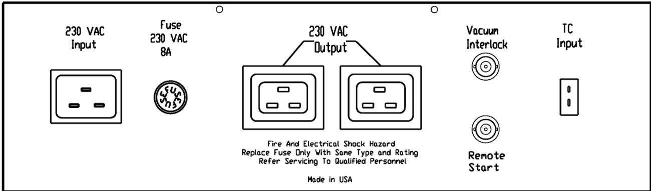
*Figure 3: BC-3 Back Panel 230V*
