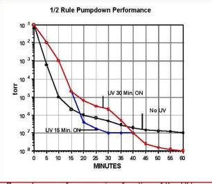
Pumpdown performance is a function of the UV power/surface area ratio and total UV exposure time. UV, properly applied, can provide either a faster pumpdown or a lower ultimate pressure.
