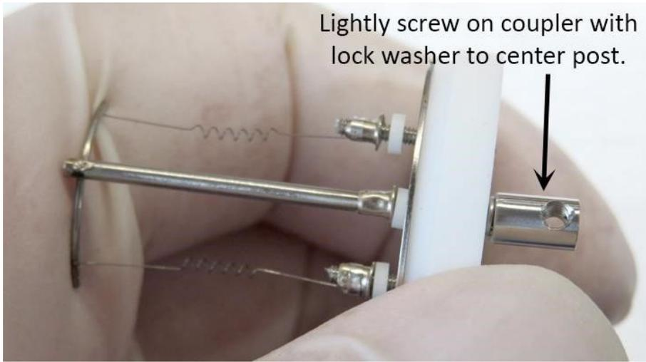
Lightly screw on coupler with lock washer to center post.
