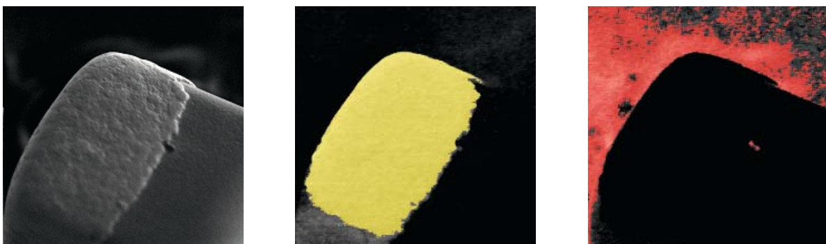
Figure A. (From L to R) SED image, tin assigned to yellow, carbon assigned to red
