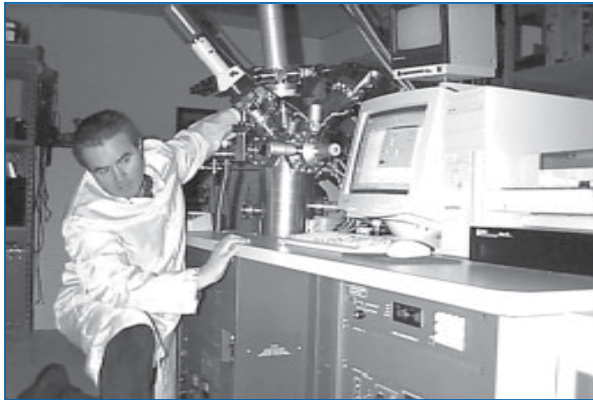
Bleeding the gas in can be difficult without a TVC remote meter
